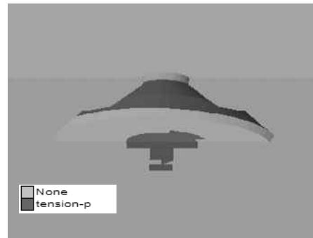
Figure 14. Plastic zone around the cave.
