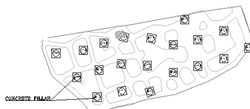
Figure 2. The layout of concrete pillars between remained pillars in Fetr6 underground mine (Faryab Co. 2008).
