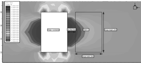
a. Horizontal stress distribution after extracting stope 1
