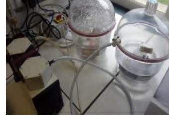
Figure 4: Experimental setup of vacuum water saturation
