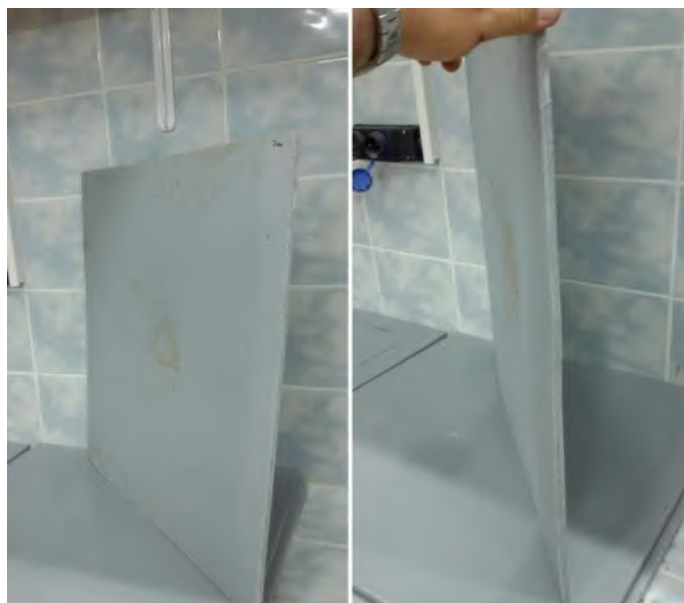
Figure 2. An elastically deformed TSL slab that had 80 mm deflection (Komurlu and Kesimal, 2017)
