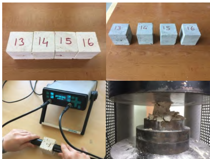
Fig. 2. Exposure of the samples to temperature and the UCS test.
