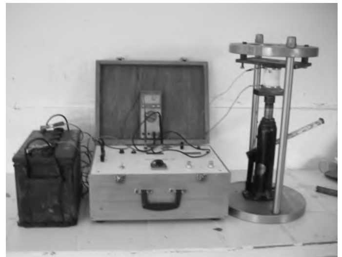
Figure 1. Resistivity measurement system.
