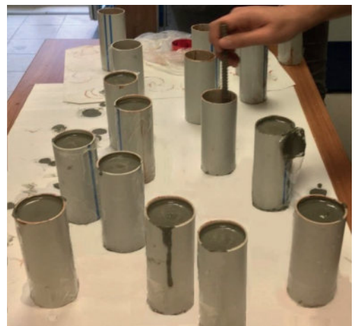
Figure 1. Preparation of UCS test specimens
