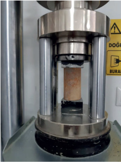
Figure 2. The UCS test
