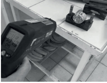
Fig. 3 The measurement of surface temperature of the specimens with an infrared gun
