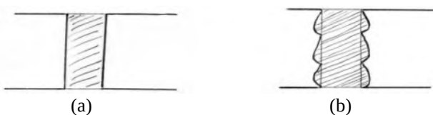
Figure 8 : Groove made by the cutter in the case of a ductile (a) and brittle (b) modes.
