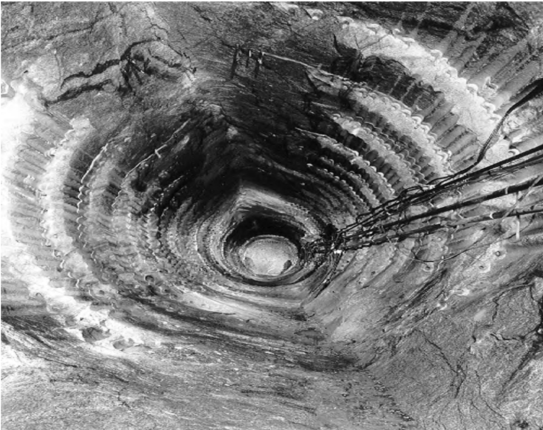
Figure 4: Shape of a circular test tunnel following the brittle failure (Picture from The Underground Research Laboratory, Pinawa, Manitoba, Canada).
